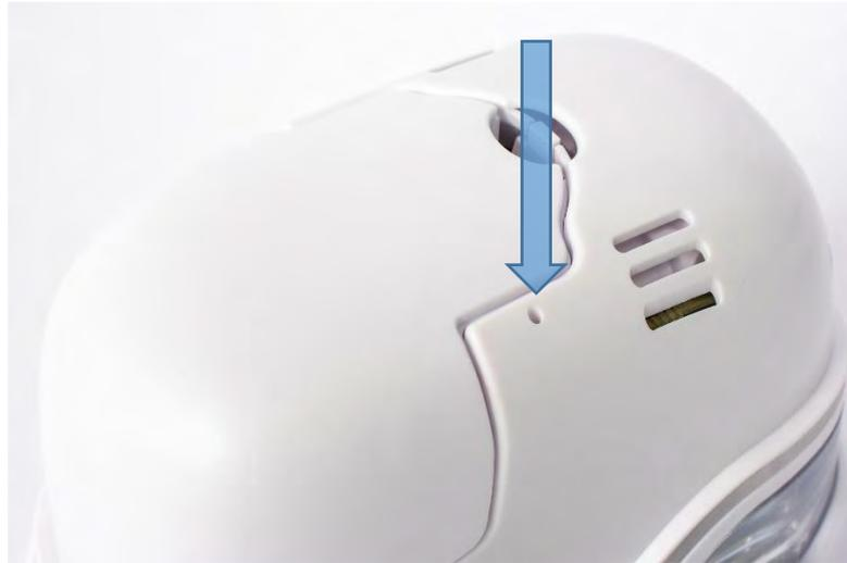
Fig. 52: Opening for device reset
