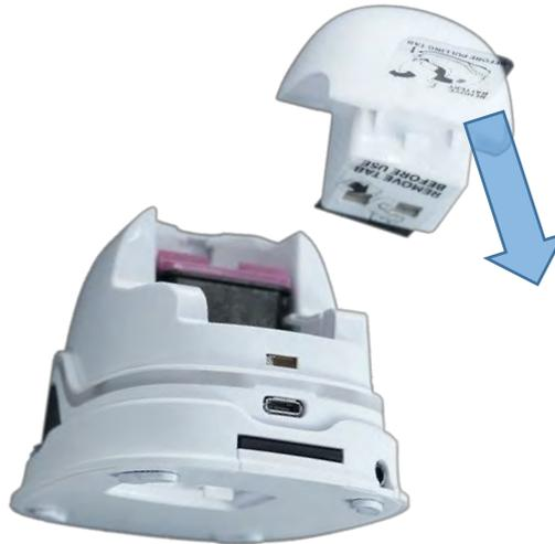
Fig. 10: Battery contact insulating tape
