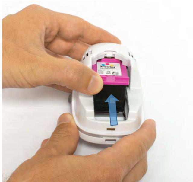
Fig. 13: Insert ink cartridge
